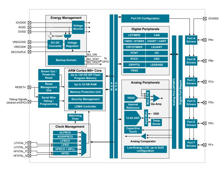
Figure 3.1. Detailed EFM32TG11 Block Diagram
