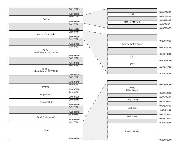
Figure 3.2. EFM32TG11 Memory Map — Core Peripherals and Code Space
