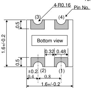
[Recommended PCB pad dimensions] Unit: mm
