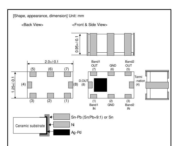
Note 1) "typ" is used where no dimensional tolerance applies.
