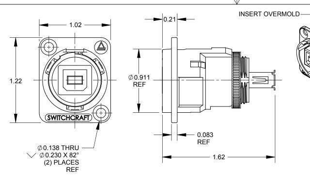
USB "A" CONNECTOR RETAINING NUT -USB "B" CONNECTOR STANDARD E SERIES HOUSING SEE TABLE FOR FINISH
