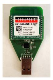
The Synapse SN132 SNAPstick USB module does not provide access to the entire range of GPIO pins available through the SN171 Proto Board. Instead, it provides a simple and compact way to connect a PC running Portal to a SNAP network.
