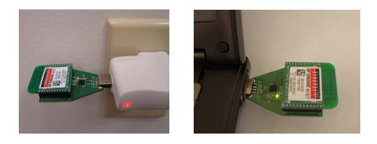
*Note:* The Portal software does not need to be installed for the SNAPstick to draw power from a PC's USB port.
