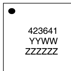
Figure 15. Top Marking Specification
