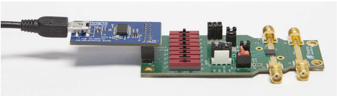
Figure 12 • USB Interface Board Connected to the Evaluation Board for Latched Parallel and Serial Programming
