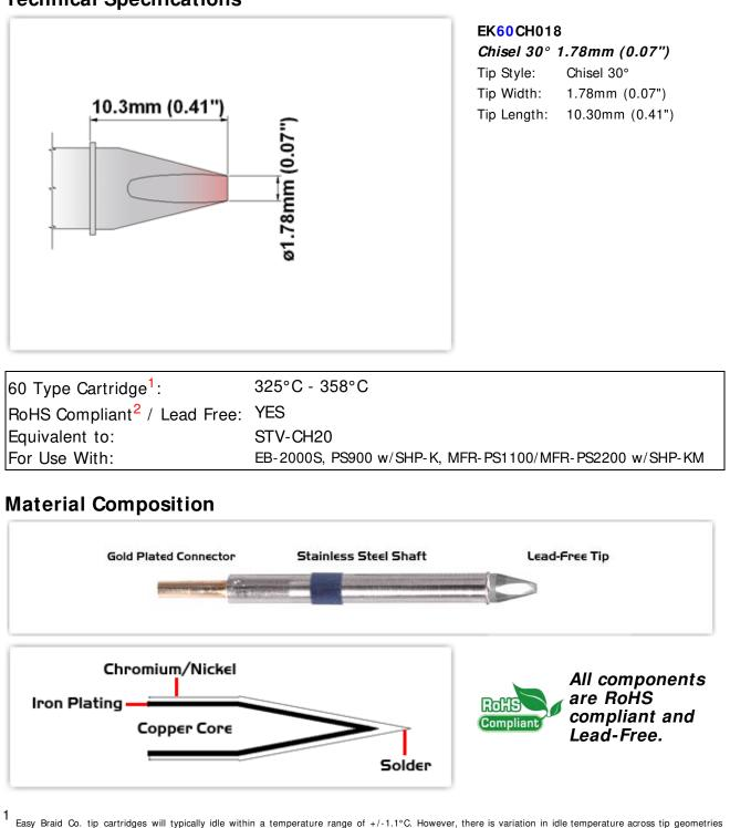
geometry of a tip will have an influence on the tip idle within a temperature arise of a transfer on the temperature across the geometries from 0.25mm fine point tip to 5mm chisel. The length and geometry of a tip will have an influence on the tip idle temperature. To accurately measure idle temperature it will depend greatly on the measurement method, technique and equipment used. Two different methods or the use of alternative equipment will produce different test results.
