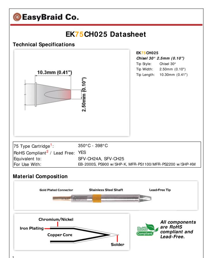
Easy Braid Co. tip cartridges will typically idle within a temperature range of +/-1.1°C. However, there is variation in idle temperature across tip geometries within an individual temperature series. Easy Braid Co. offers a wide variety of tip geometries from 0.25mm fine point tip to 5mm chisel. The length and geometry of a tip will have an influence on the tip idle temperature. To accurately measure idle temperature it will depend greatly on the measurement method,
