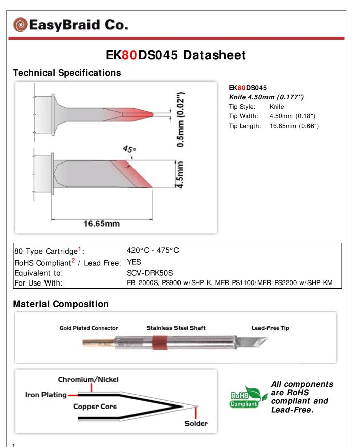
Easy Braid Co. tip cartridges will typically idle within a temperature range of +/-1.1°C. However, there is variation in idle temperature across tip geometries within an individual temperature series. Easy Braid Co. offers a wide variety of tip geometries from 0.25mm fine point tip to 5mm chisel. The length and geometry of a tip will have an influence on the tip idle temperature. To accurately measure idle temperature it will depend greatly on the measurement method,
