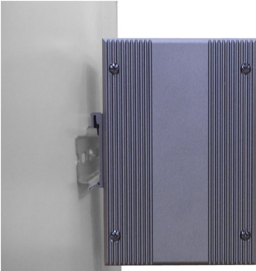
Figure 2.7: Installation to DIN-rail Step 2
