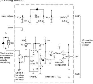
Note: This is the reference circuit which drives the PIR motion sensor. Install a noise filter for applications requiring enhanced detection reliability and noise withstanding capability.
