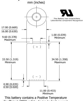
Coefficient (PTC) safety device to limit current during short circuit conditions.
