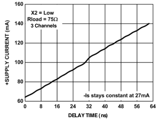
FIGURE 8. POSITIVE SUPPLY CURRENT vs DELAY TIME
