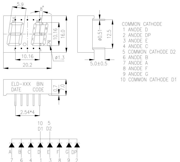
**Notes:** 1.All dimensions are in millimeters, tolerance is 0.25mm unless otherwise noted.
