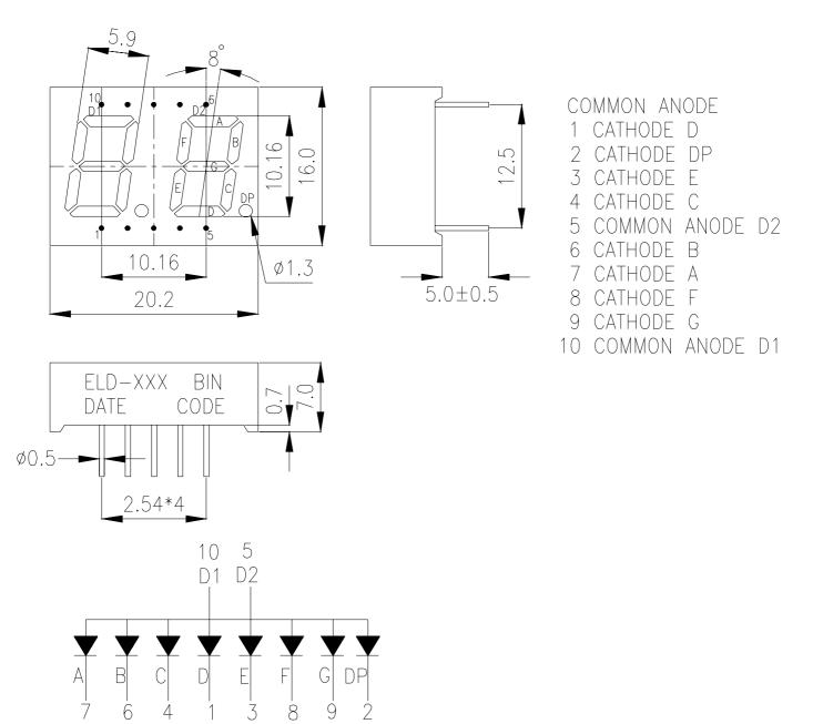
Notes: 1.All dimensions are in millimeters , tolerance is 0.25mm unless otherwise noted.2.Above specification may be changed without notice.
