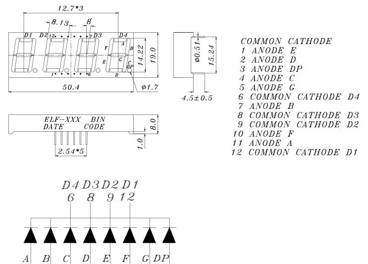
Notes: 1.All dimensions are in millimeters, tolerance is 0.25mm unless otherwise noted.
