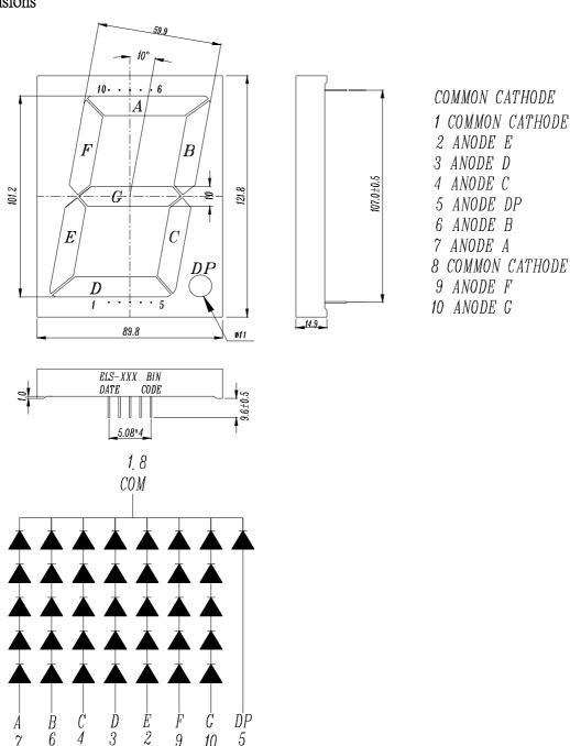
**Notes:** 1. All dimensions are in millimeters, tolerance is 0.25mm unless otherwise noted.
