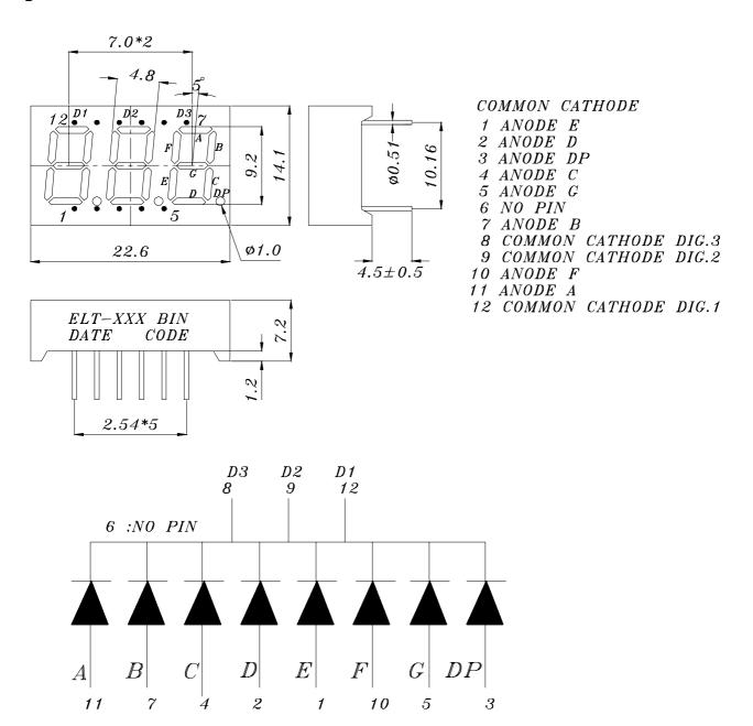
**Notes:** 1. All dimensions are in millimeters, tolerance is 0.25mm unless otherwise noted.
