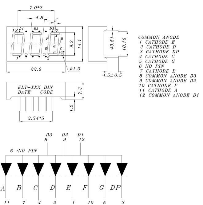
Notes: 1.All dimensions are in millimeters, tolerance is 0.25mm unless otherwise noted.
