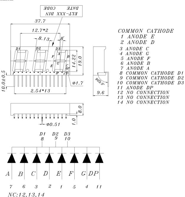
**Notes:** 1. All dimensions are in millimeters, tolerance is 0.25mm unless otherwise noted.
