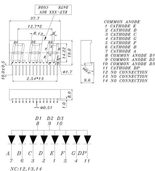
**Notes:** 1. All dimensions are in millimeters, tolerance is 0.25mm unless otherwise noted.
