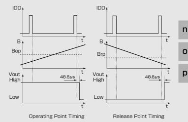
This Hall IC's output is held as internal data just before the internal circuit turns OFF (IDD OFF). And after 48.8  $\,\mu$ s, the output changes. Note) 48.8  $\,\mu$ s in figures is typical value
