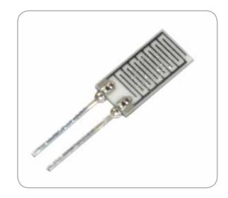
The EMD-4000B is a bulk resistance-type humidity sensor based on the impedance change of a thinfilm polymer due to water vapor absorption. The polymer is deposited on Bismuth alloy terminals, which are set on a ceramic substrate. The sensor is excited by a low voltage alternating current and the impedance measured as a function of relative humidity.
