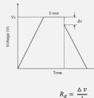
$R_d$  is the ESR<sub>DC</sub> ( $\Omega$ ); Where  $\Delta v$  is the voltage drop for 10ms (V); I is the discharge current (A).
