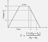
Where  $v_1$  is the measurement starting voltage,  $0.8 \times V_R$  (V);  $v_2$  is the measurement end voltage,  $0.4 \times V_R$  (V);  $t_1$  is the time from discharge start to reach  $v_1$  (s);  $t_2$  is the time from discharge start to reach  $v_2$  (s); I is the absolute value of the discharging current (A).
