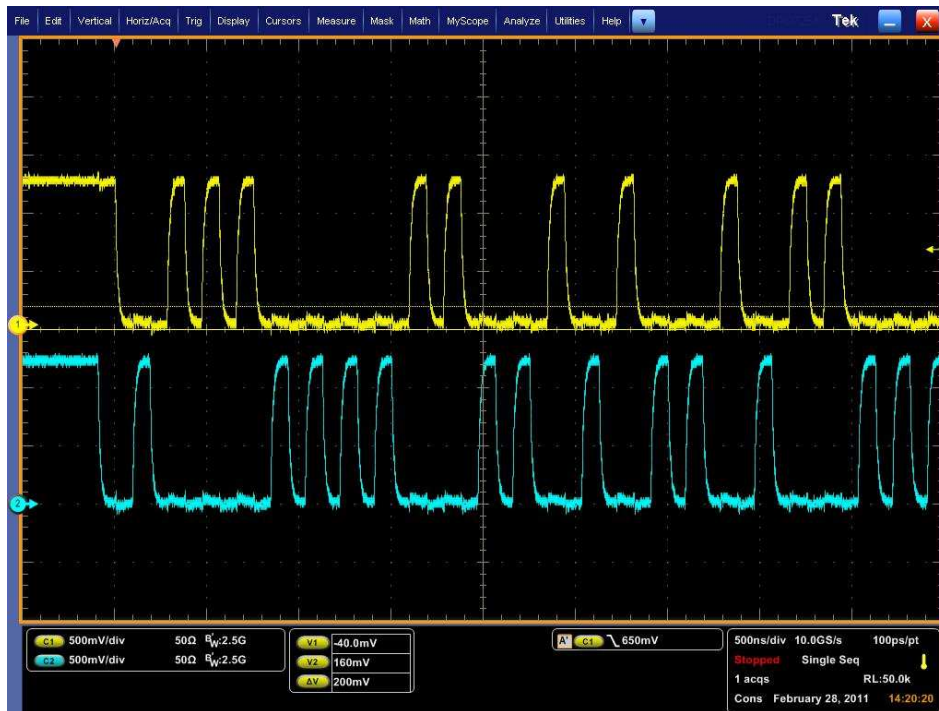
Figure 8. EMI4163MU MIPI D-PHY LP Mode Measured Results
