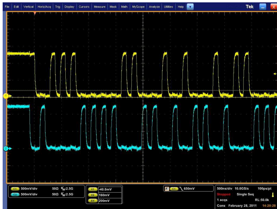
Figure 5. EMI4172 MIPI D-PHY LP Mode Measured Results
