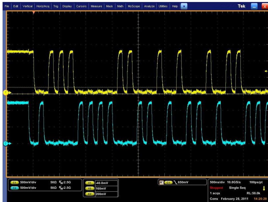
Figure 8. EMI4182 MIPI D-PHY LP Mode Measured Results
