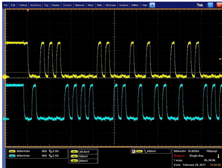
Figure 8. EMI4184 MIPI D-PHY LP Mode Measured Results
