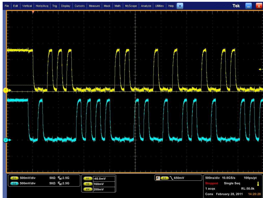
Figure 5. EMI4193 MIPI D-PHY LP Mode Measured Results
