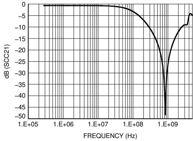
**Figure 3. Typical Common Mode Attenuation vs. Frequency**
