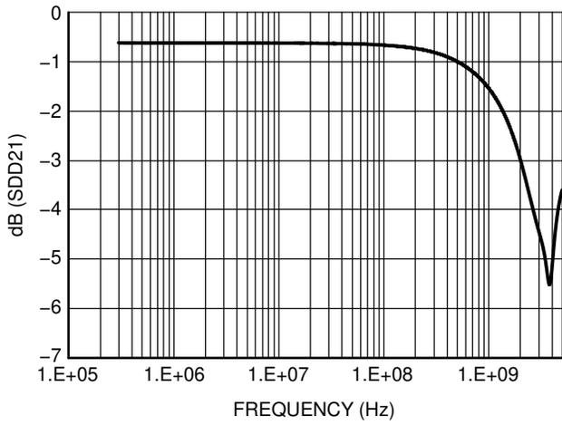
**Figure 2. Typical Differential Mode Attenuation vs. Frequency**
