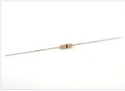
A zerohm jumper looks like a resistor with one black stripe.
