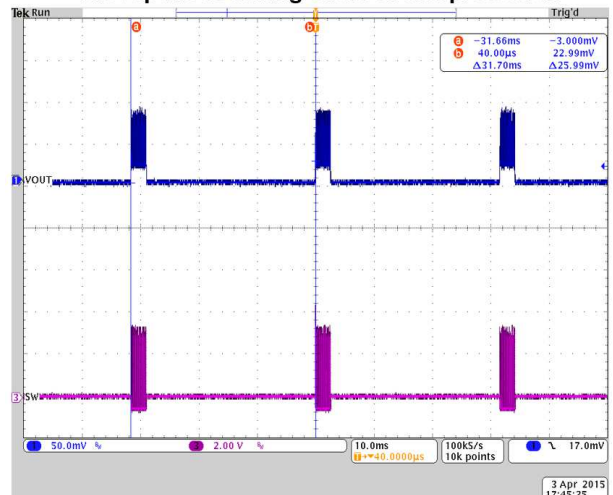
Hiccup mode during short-circuit protection
