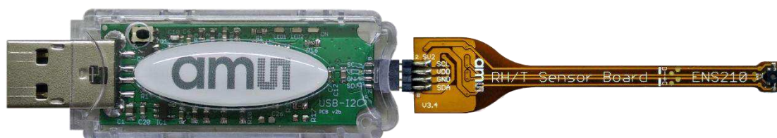
Figure 2 ENS210 Sensor Board with USB-I2C Dongle
