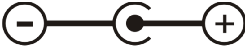
Figure 3 Barrel Connector J7 Polarity
