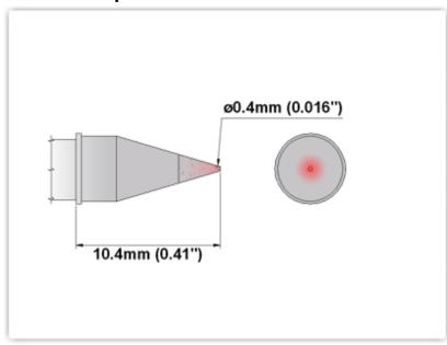
EP75 C004 Conical 0.40mm (0.016")
