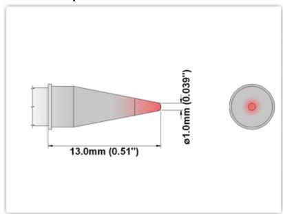
EP75 C010 Conical 1.00mm (0.04")
