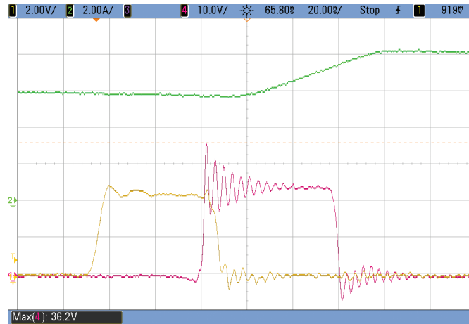
Figure 4: Typical Waveforms for V_{IN} = 24V to 1.2V/7A (1000kHz) Buck converter CH1: V_{pwm} Input voltage – CH2: (I_{out}) Switch node current – CH4: (V_{out}) Switch node voltage
