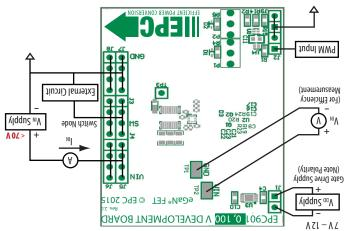
Figure 2: Proper Connection and Measurement Setup
