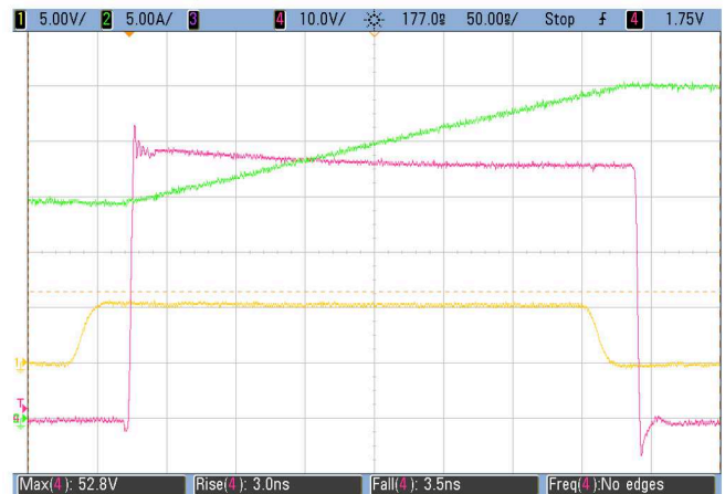
Figure 4: Typical Waveforms for V_{IN} = 48 V to 5 V/25 A (300 kHz) Buck converter CH1: ( V_{PWM} ) Input logic signal – CH2: ( I_{OUT} ) Output inductor current – CH4: ( V_{OUT} ) Switch node voltage
