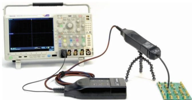
Figure 4: Tektronix IsoVu measurement setup.
