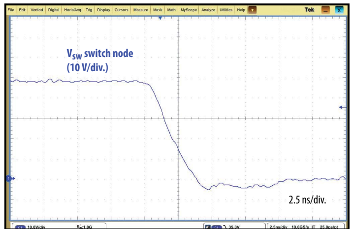
Figure 4: Typical switch node waveforms taken at 48 V IN to 12 V OUT /50 A OUT
