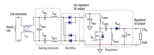
Figure 2: Schematic diagram of the EPC9513 demo board.
