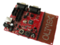
Olimex - SAM7-P DEVELOPMENT FOR AT91SAM7S ARM7TDMI-S MC
