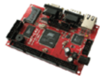
Olimex - SAM7-L DEVELOPMENT FOR AT91SAM7E ARM7TDMI-S MC
