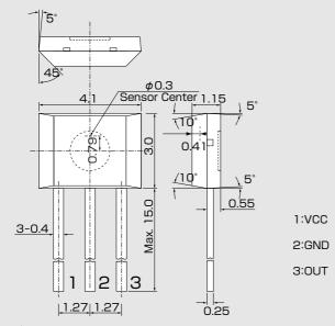
Note 1) The sensor center is located within the  $\phi$ 0.3mm circle.
