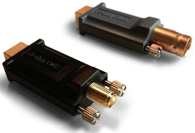
The dongles give users the flexibility to determine the best cable lengths for their applications. The transceiver contains an equalizer that is fully adaptive that adjusts to a variety of cable lengths as well as age and environmental conditions like temperature, without any need for programming. The dongles have a standard 1394b 9-pin connector on one end and a 75Ω BNC or 50Ω SMA connector on the opposite end.
