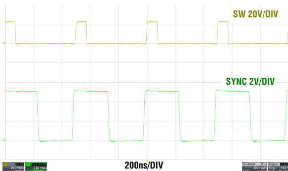
FIGURE 39. SYNC AT 1A LOAD, PWM
