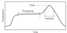
For soldering (Example: Sn/Pb)
