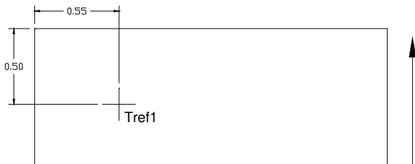
Figure 18. Case ( T_{REF} ) Temperature Measurement Location (top view).
