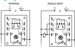
2-3 & 7-6 are Normally Open Contacts (NO)2-4 & 7-5 are Normally Closed Contacts (NC)
